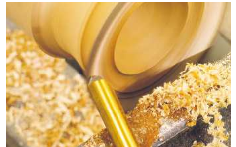
▲ Pic.4 The final finishing cuts are the other way with a 6mm bowl gouge; as you go thin a push cut gives you more chance of keeping the bark on
